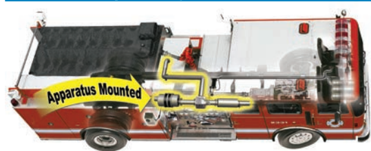
Figure 6.13 — An apparatus-mounted exhaust capture system.
