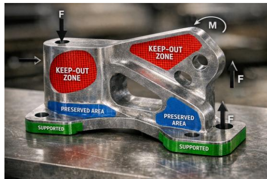
Figure 2. Design space setup showing applied loads, supports, preserved areas, and keep-out zones.
